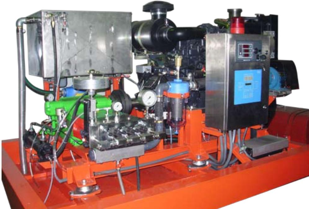
U H P (Ultra High Pressure) units designed for special surface treatments (descaling, hydrodemolition, surface preparation, etc.) with manual spray gun or with the use of a robot.
