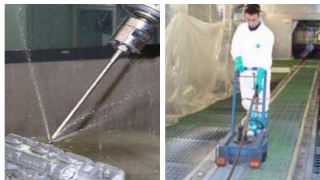
Cleaning of lube oil channels in engine blocks, heads and over-heads, axle shafts, two-stroke engines cylinders, deburring of aluminium castings, grille cleaning in spray booths, and plastic bumpers frames
