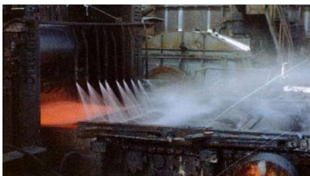
Descaling of slabs, heat exchangers, ingot moulds, blast furnace cooling systems, coke oven doors, absorption filters, pipelines, tanks, eyeclean ducts, etc.
